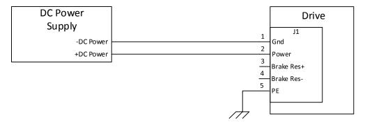
Figure 10: Power supply connection to the drive
