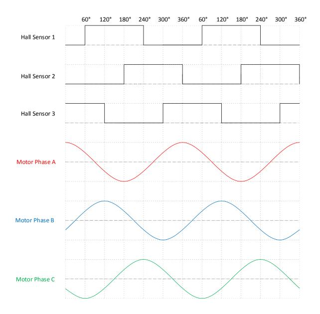
Figure 3: Sinusoidal commutation with Hall sensor feedback
