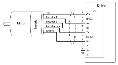
Figure 15: Single-ended encoder connection to the drive
