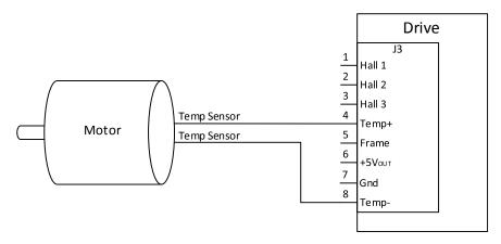
Figure 17: Temperature sensor connection to the drive
