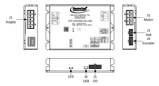
Figure 9: Drive connector layout
