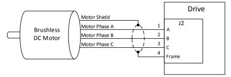
Figure 11: Brushless DC motor connection to the drive
