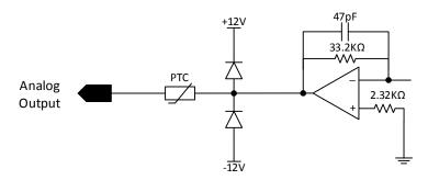
Figure 23: Analog output circuit
