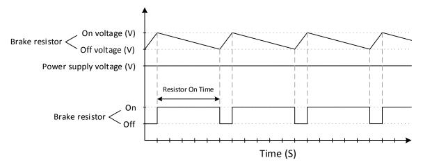
Figure 25: Brake resistor operation graph
