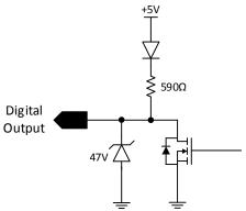
Figure 21: Digital output circuit
