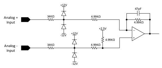
Figure 22: Analog input circuit
