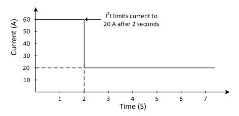
Figure 7: I<sup>2</sup>t algorithm example
