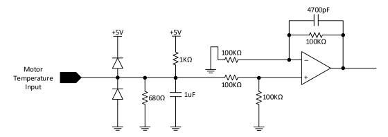
Figure 18: Temperature sensor signal input circuit
