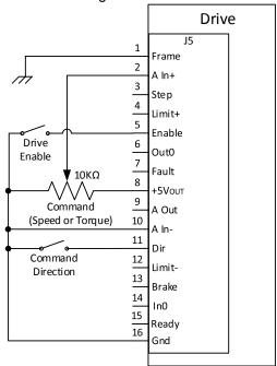
Figure 19: Minimum drive I/O connections needed to operate BLDC and PMDC motor
