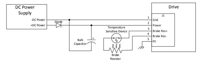
Figure 26: External brake resistor and bulk capacitor connection to the drive
