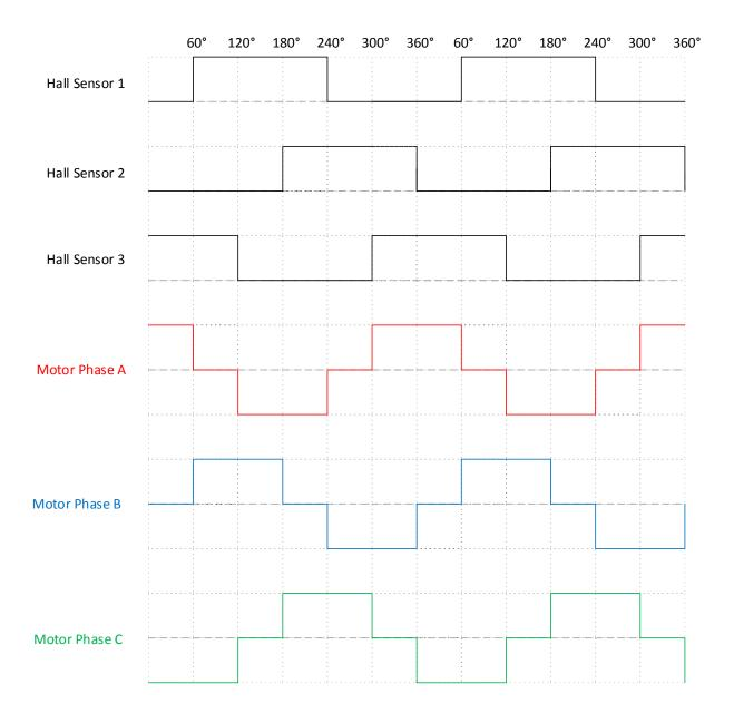
Figure 2: Trapezoidal Commutation with Hall sensor feedback
