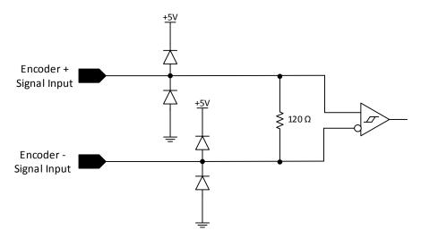
Figure 16: Encoder signal-ended input circuit
