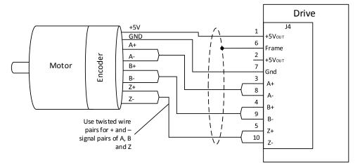
Figure 14: Differential encoder connection to the drive
