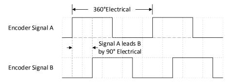
Figure 4: Encoder feedback signal
