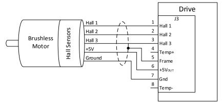
Figure 12: Hall sensor connection to the drive
