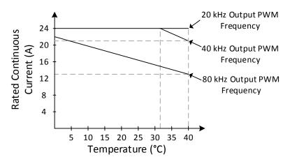
Figure 6: Drive temperature derating at 80VDC
