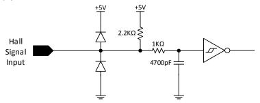
Figure 13: Hall sensor signal input circuit
