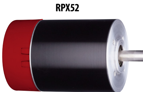
RPX52 1,650mNm Peak Torque with 435mNm of continuous torque and 130W of power at 2,900RPM
